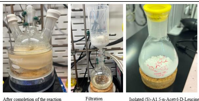
Figure 3.2.6. Representative pictures of scale-up synthesis of ( S )- A1.5-NADL on 10 g scale
